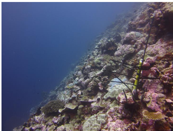
Figure 32. A subsurface temperature recorder (STR) secured to the reef at 17.5 m on Salomon Atoll.
