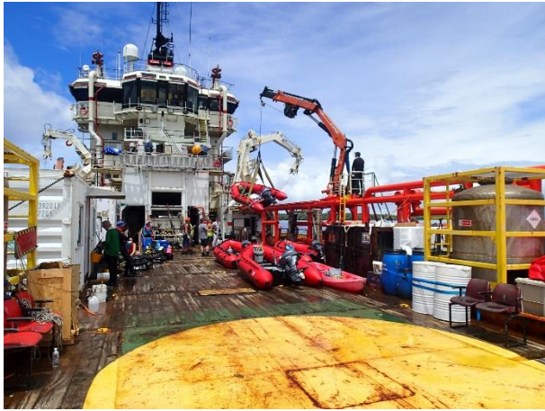
Figure 40. Deck container lab (left) provides an air conditioned dry work space on deck (right)
