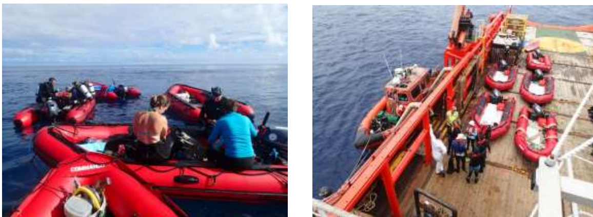
Figure 39. 5 x 4.2m inflatable boats are used to support diving operations and are launched from the deck of the BPV Grampian Frontier. The ship's Daughter craft (right) is used when conditions do not allow the launch of the inflatable boats using the deck crane.
