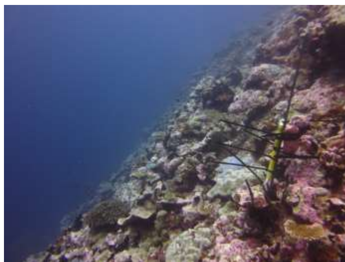
Figure 32. A subsurface temperature recorder (STR) secured to the reef at 17.5 m on Salomon Atoll.
