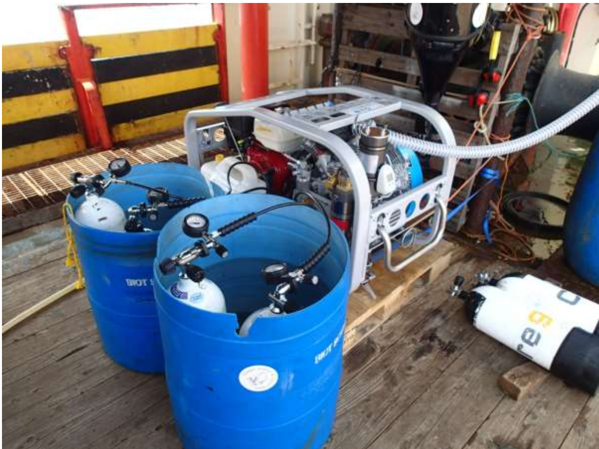
Figure 38. New Bauer Mariner 320B compressor capable of filling 4 cylinders simultaneously in under 30 minutes. The compressor stops automatically when the cylinders are full, and filters are drained automatically into an integral disposal tank.
