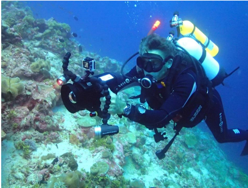
Figure 26. High Definition camera in housing with wide angle port, LED lights, laser scale and Go-Pro camera recording digital images every 30 seconds.
