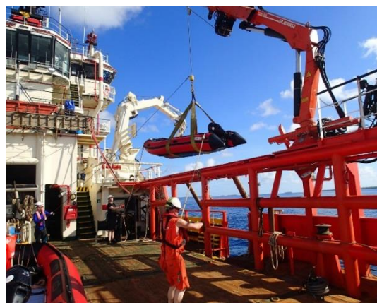
Figure 63. Lifting dive boats with crane & strops
