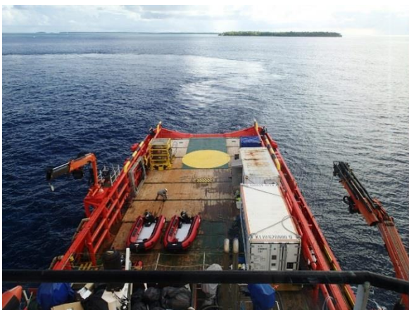
Figure 62. Aft deck area and cranes with freezer and lab containers and fuel stores at stern
