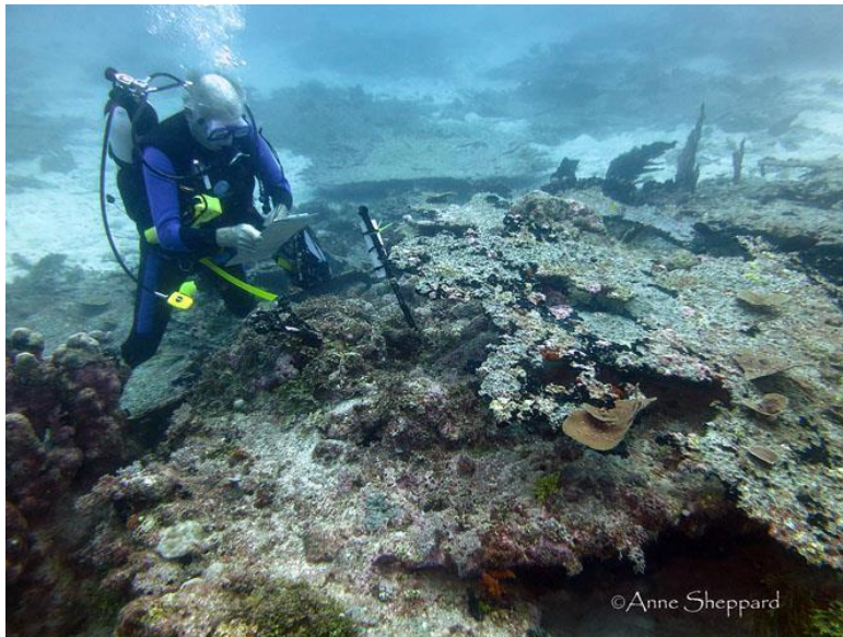
Figure 21. New temperature logger in protective pipe attached to the stake at 15 m depth in Peros Banhos lagoon. The surrounding corals are all dead at this location (the live plate in foreground is a sponge).
