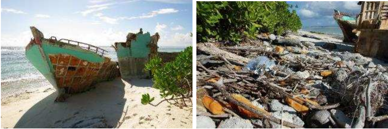
Fishing vessel on NW DG shore, November 2018. The vessel has moved and changed orientation but the two largest parts of the hull remain intact. Waste matter from the vessel continues to spread along the shore, including large volumes of light, hardened polyurethane foam (right).
